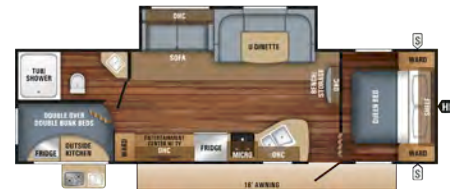
JAY FLIGHT SLX | 284BHS OPTION A Ext. Lgth: 33' 5" Ext. Ht: 132" Unloaded Wt. (lbs): 6,140 Sleeps: 6-8
