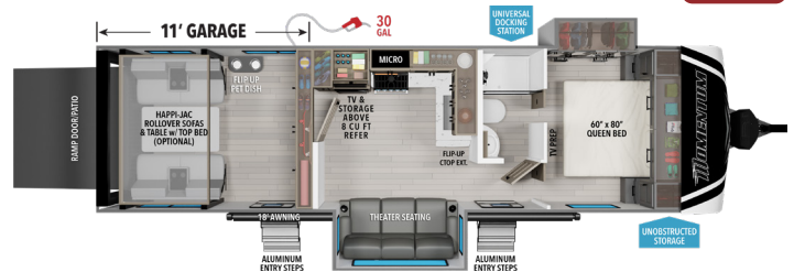
29GS 11' GARAGE UVW 1 HITCH 1 GVWR LENGTH 2 HEIGHT CAPACITY TBD TBD 13,000 34' 6" 12' 4" 90 78 39
