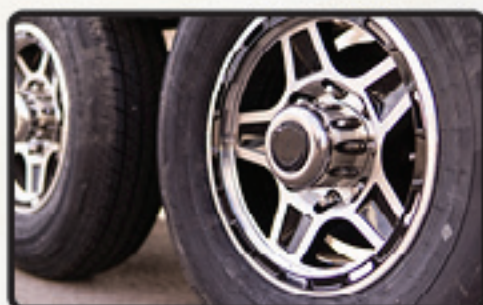
8 LUG ALUMINUM RIMS RATED AT 110 PSI (APPROVED FOR G RANGE)
