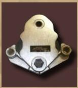
SuperLites Equa Flex suspension is constructed from specially formulated rubber that absorbs vibration from road bumps, holes and cracks.
