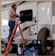
Seal Tech Air Pressure Test
