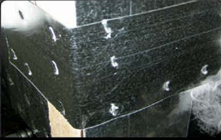
EVERLAST® Cross Banded Construction
