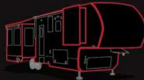
Utilizing Mylar Tape and Die-Cut Seals at ALL critical seams (roof to sidewall, floor to sidewall and backwall to sidewall).
