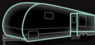
4 protective layers (mylar tape, 2-layers of PVC foam, and a final silicone cap seal) line the perimeter of the coach for ultimate protection from the elements.
