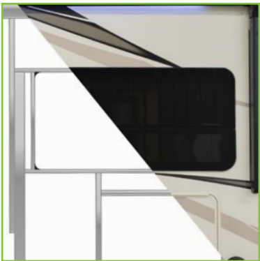
Aluminum Framing Around Windows in Sidewall
