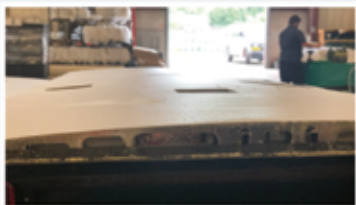
ONE PIECE WRAPPED FIBERGLASS ROOF NO SEAMS FROM FASTENERS ON RADIUS
