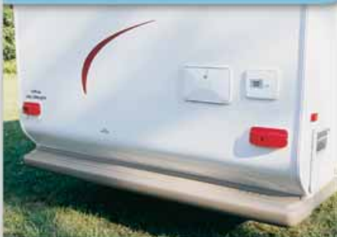
The molded ABS rear bumper cover creates a smooth, attractive surface.
