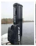
FENDER HANGER Bracket is screwed into the side rail to conveniently place fenders for the dock.
