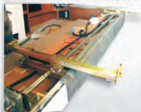
Dual Ram Rack and Pinion Slide Assembly in All Slide Outs
