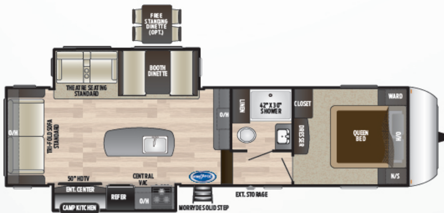
299RLDS | Two-slide, rear entertainment, island kitchen, camp kitchen, re-designed bedroom Weight: 9020 LBS. | Length: 33' 0"
