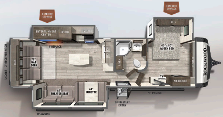
2906BS REAR LIVING UUV: 8559 HITCH: 1100 AXLE: 7400 CCC: 1341 LENGTH: 35' 5" ULTRA LITE WIDTH: 8' HEIGHT: 11' 3" FRESH: 54 gal GRAY: 45 gal BLACK: 45 gal
