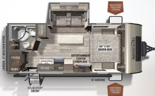
2205S REAR LIVING UVW: 5004 HITCH: 530 AXLE: 4415 CCC: 1686 LENGTH: 23' 10" MINI LITE WIDTH: 8' HEIGHT: 10' 11" FRESH: 54 gal GRAY: 30 gal BLACK: 30 gal
