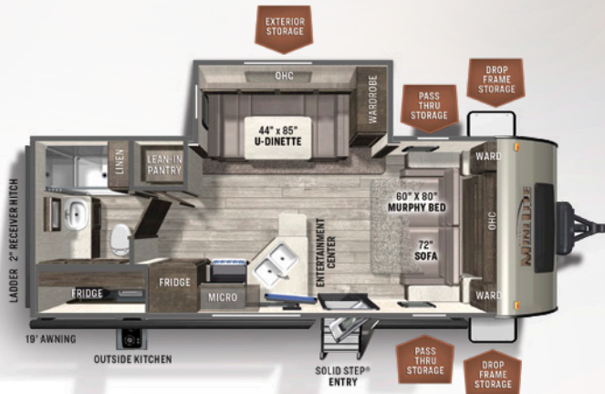
2507S MURPHY BED UVW: 5471 HITCH: 625 AXLE: 4787 CCC: 1314 LENGTH: 25' 10" MINI LITE WIDTH: 8' HEIGHT: 10' 11" FRESH: 54 gal GRAY: 30 gal BLACK: 30 gal
