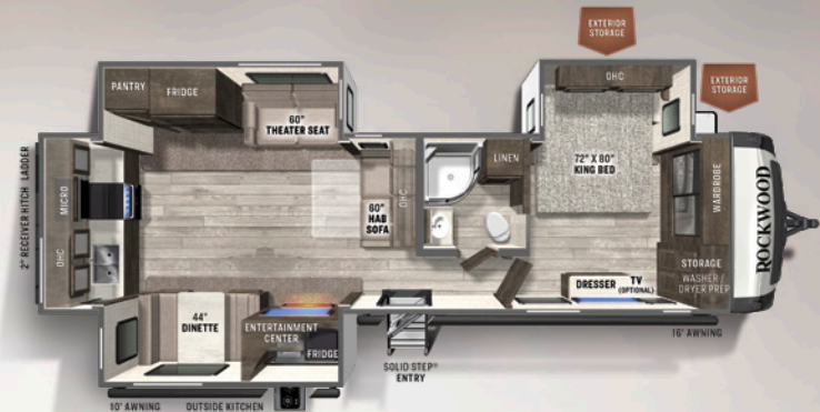
8332SB REAR KITCHEN SIGNATURE U/VW: 9444 HITCH: 1130 AXLE: 8255 CCC: 1686 LENGTH: 36' 8" WIDTH: 8' HEIGHT: 11' 7" FRESH: 54 gal GRAY: 110 gal BLACK: 50 gal
