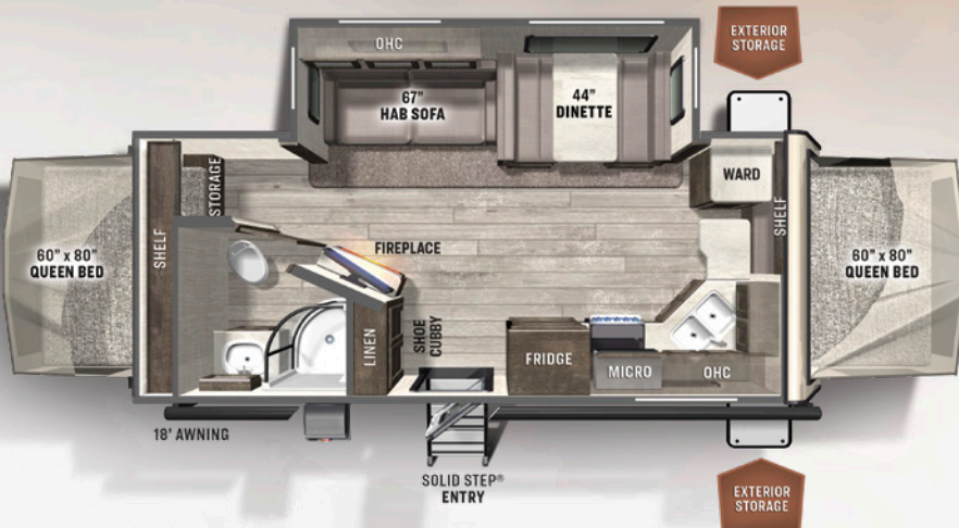
23FK EXPANDABLE UUV: 5528 HITCH: 720 AXLE: 4770 LENGTH: 24'10" OPEN LENGTH: 29'7" ROO CCC: 1352 WIDTH: 8' HEIGHT: 10'11" FRESH: 54 gal GRAY: 30 gal BLACK: 30 gal
