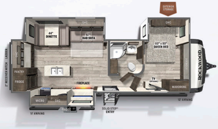
2720IK REAR KITCHEN UUV: 8324 HITCH: 1035 AXLE: 7230 CCC: 1511 LENGTH: 33' 1" ULTRA LITE WIDTH: 8' HEIGHT: 11' 3" FRESH: 54 gal GRAY: 90 gal BLACK: 45 gal
