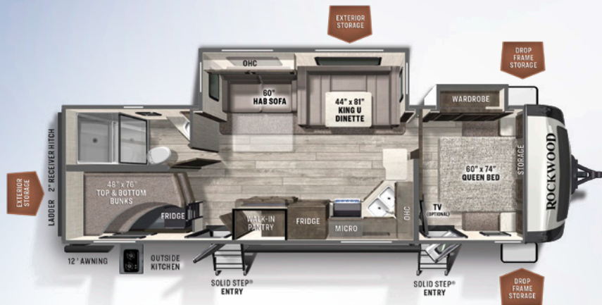
2706WS BUNK HOUSE UUV: 7310 HITCH: 921 AXLE: 6330 CCC: 1411 LENGTH: 32' 10" ULTRA LITE WIDTH: 8' HEIGHT: 11' 2" FRESH: 54 gal GRAY: 90 gal BLACK: 45 gal
