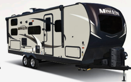
2506S FRONT KITCHEN MINI LITE U/VW: 5281 HITCH: 644 AXLE: 4510 CCC: 1523 LENGTH: 25'11" WIDTH: 8' HEIGHT: 10'11" FRESH: 54 gal GRAY: 60 gal BLACK: 30 gal
