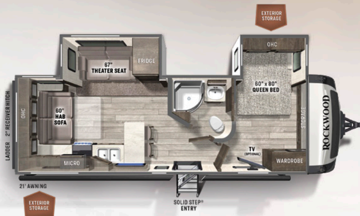
2613BS REAR LIVING UVW: 6614 HITCH: 915 AXLE: 5640 CCC: 2101 LENGTH: 29' 9" ULTRA LITE WIDTH: 8' HEIGHT: 11' 2" FRESH: 54 gal GRAY: 90 gal BLACK: 45 gal
