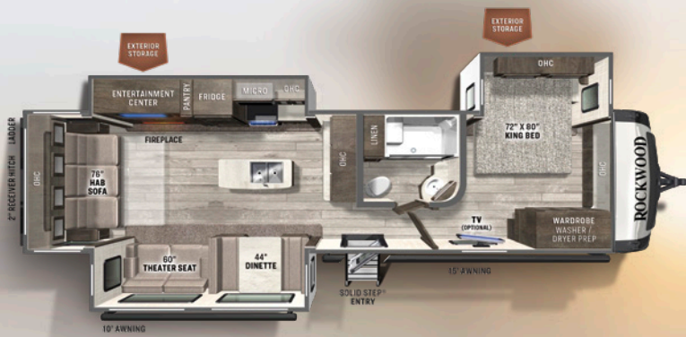
8337RL REAR LIVING SIGNATURE U/VW: 9209 HITCH: 1315 AXLE: 7835 CCC: 2106 LENGTH: 36' 8" WIDTH: 8' HEIGHT: 11' 7" FRESH: 54 gal GRAY: 120 gal BLACK: 50 gal
