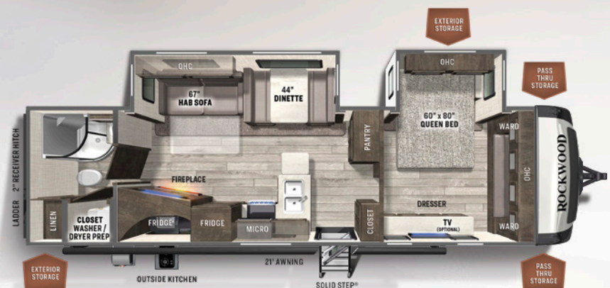
2912BS REAR LIVING UUV: 7854 HITCH: 952 AXLE: 6843 CCC: 1898 LENGTH: 35' 2" ULTRA LITE WIDTH: 8' HEIGHT: 11' 2" FRESH: 54 gal GRAY: 90 gal BLACK: 45 gal
