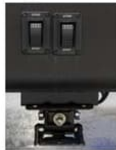
4 power stabilizer jacks, each with its own independent motor.
