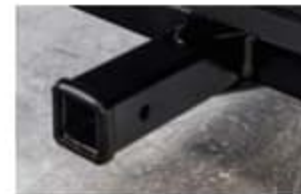
2-Inch accessory hitch is integrated into the frame.
