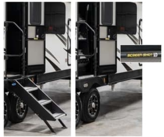
All SportTrek Tourings feature a solid flip-up step and friction-hinged entry door with Screen Shot screen door.
