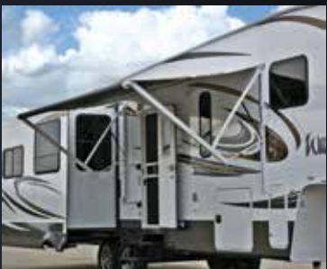
Easy to use "one-touch" electric awnings (with fully adjustable arms) allow for quick setup and retraction at your camp site.
