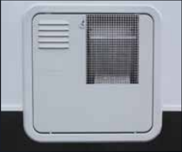
The 10 gallon DSI gas/electric quick recovery water heater (16.2 gallons per hour) provides an abundant supply of hot water and is great while dry-camping too.
