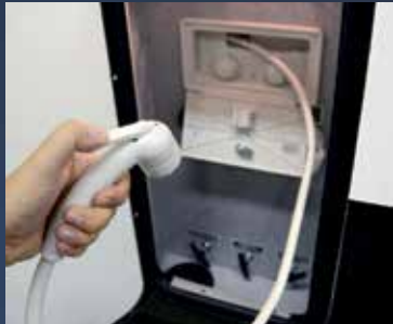
A fully enclosed and lighted docking center, including outside shower and black tank flush, puts all your dump valves and connections in one place.
