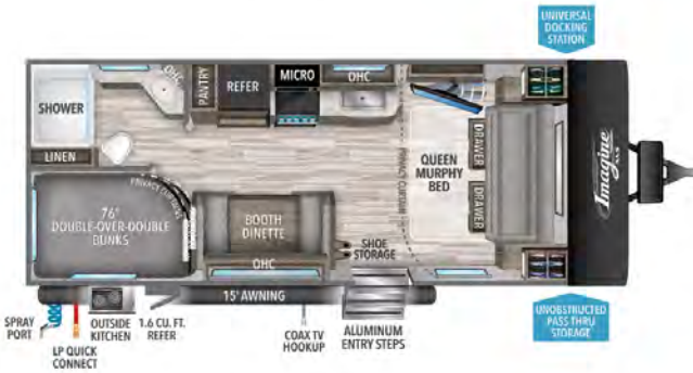
21BHE UVW' 4,698 HITCH' 456 LENGTH' 24' 11" HEIGHT 10' 5" CAPACITY 43 45 37
