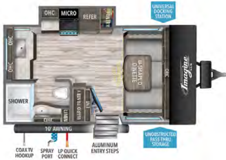
15FLE UVW' 4,036 HITCH' 418 LENGTH' 19' 4" HEIGHT 10' 5" CAPACITY 43 45 37
