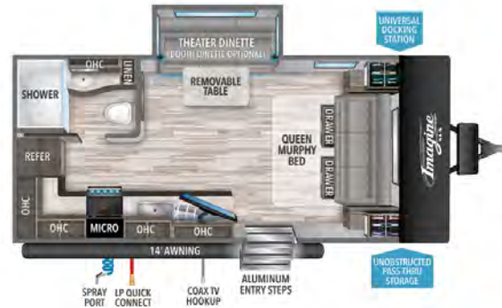
17MKE UVW' 4,674 HITCH' 480 LENGTH' 21' 11" HEIGHT 10' 5" CAPACITY 43 45 37
