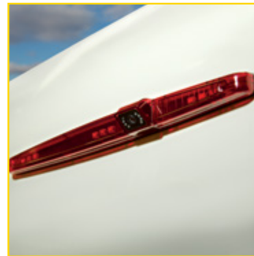
Back-up Monitor with Integrated Rear Camera
