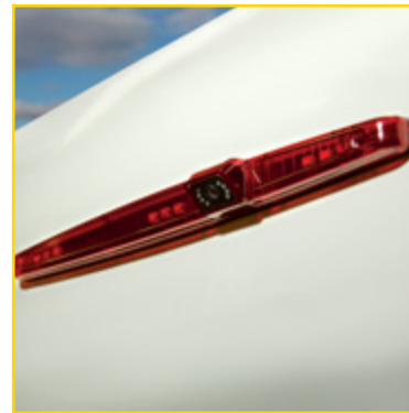
Back-up Monitor with Integrated Rear Camera
