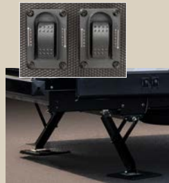
4 power stabilizer jacks, each with its own independent motor.
