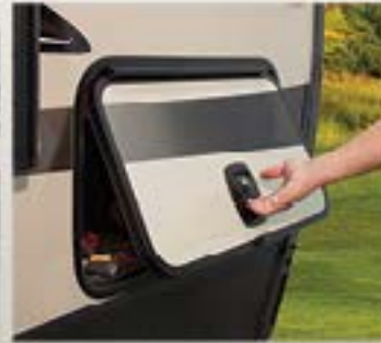
Slam Latch Garage Doors with magnetic door catches
