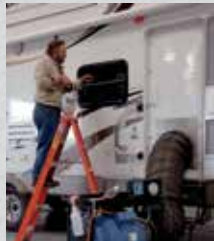
Seal Tech Air Pressure Test
