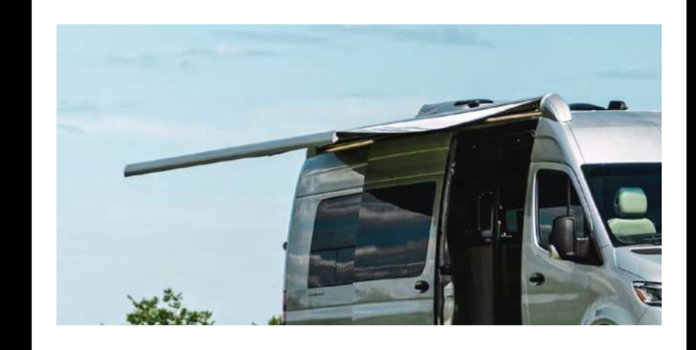
2 The powered awning extends and retracts at the push of a button.
