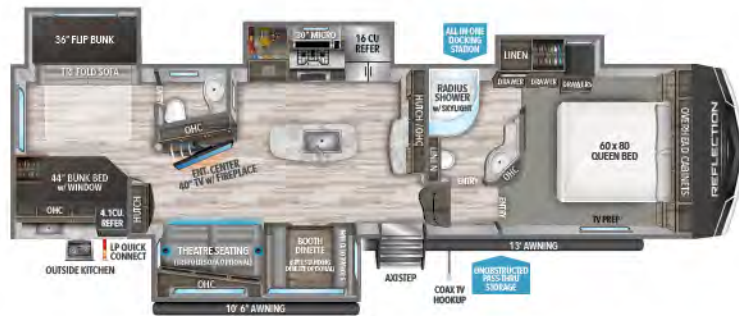
311BHS UVW 1 11,377 HITCH 1 2,316 LENGTH 2 36' 10" HEIGHT 3 12' 3" CAPACITY 74 87 87
