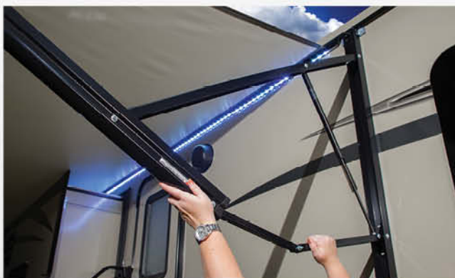
Power Awning with LED Lights
