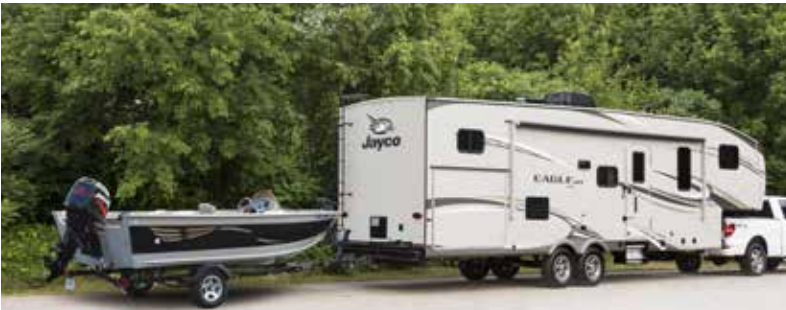
STANDARD INTEGRATED REAR 2-INCH RECEIVER HITCH WITH 300-POUND TONGUE CAPACITY AND 3,000-POUND TOW RATING (EAGLE HT ONLY)
