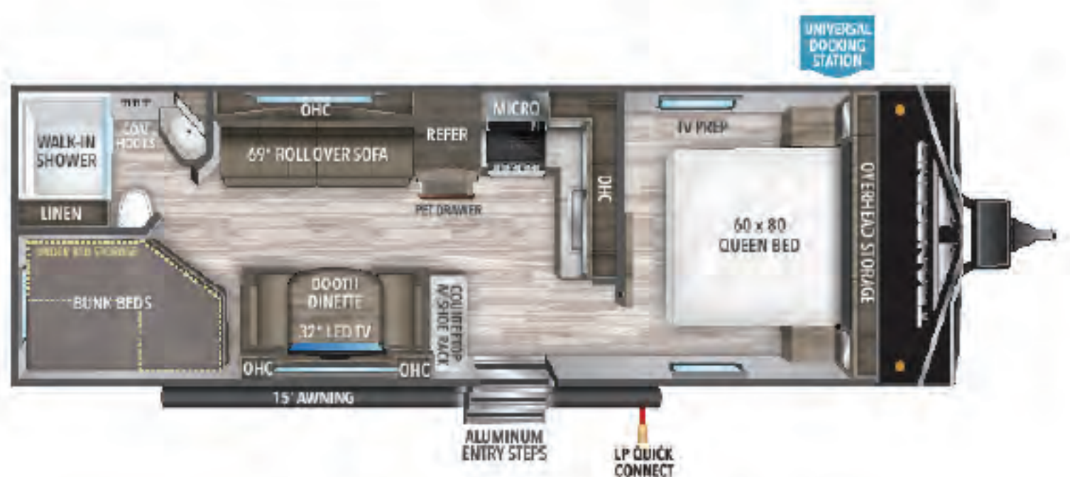
247BH UVW' 5,392 HITCH' 546 LENGTH' 29' 11" HEIGHT 11' CAPACITY 62 78 39
