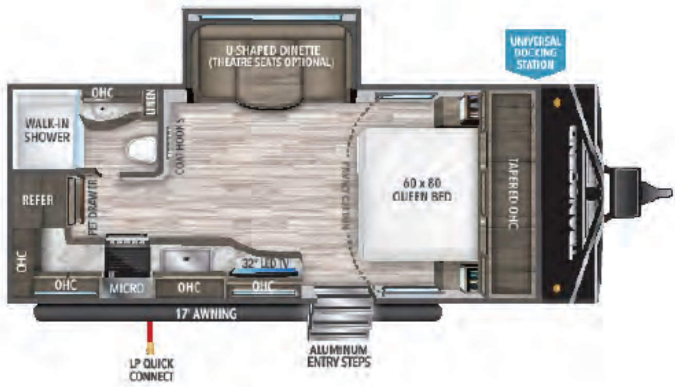
200MK UVW' 4,796 HITCH' 480 LENGTH' 24' 11" HEIGHT 11' CAPACITY 62 39 39
