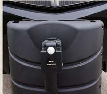
Power Tongue Jacks are standard on all Outback trailers and greatly reduce set up time.
