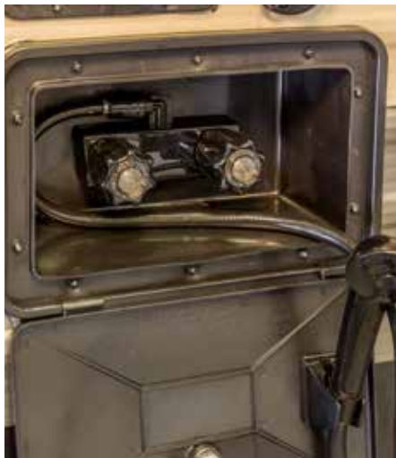
Outside Shower With Hot And Cold Water
