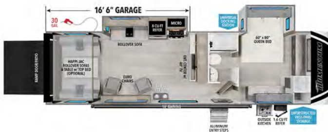
28G 16' 6" GARAGE UVW' EMPTY HITCH' GVWR LENGTH' HEIGHT CAPACITY 9,153 1,368 13,000 33' 11" 12' 4" 90 78 39
