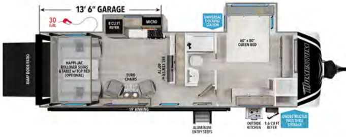
25G 13' 6" GARAGE UVW' EMPTY HITCH' GVWR LENGTH' HEIGHT CAPACITY 7,900 1,150 13,000 30' 11" 12' 4" 90 78 39
