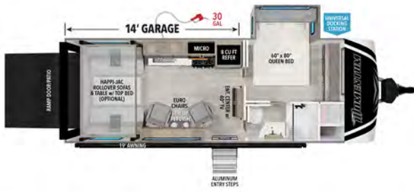
21G 14' GARAGE UVW' EMPTY HITCH' GVWR LENGTH' HEIGHT CAPACITY 6,400 920 11,000 26' 11" 12' 4" 90 74 39
