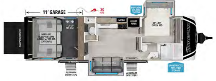
29G 11' GARAGE UVW' EMPTY HITCH' GVWR LENGTH' HEIGHT CAPACITY 9,278 1,592 13,000 33' 11" 12' 4" 90 37 39 37* * 1/2 BATH DOUBLES AS BLACK/GREY
