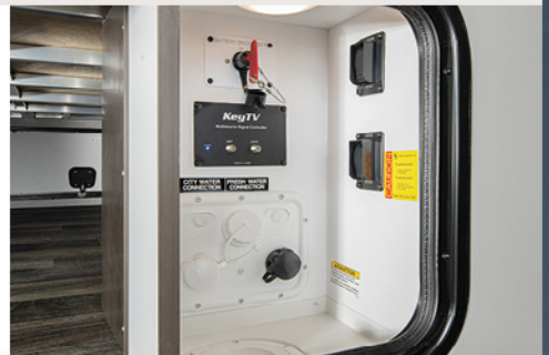
Docking Station w/ Battery Disconnect Easily accessible convenience center with water connections, KeyTV™ hookups, stabilizer jack switches, and our first ever battery disconnect.
