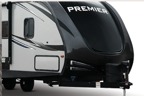
Full Fiberglass Front Cap Premier's full fiberglass front cap features Keystone's KeyShield™ five-layer paint technology that prevents cracking and fading.
