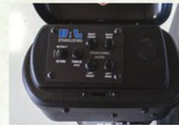
5-Point stabilizing Power Tongue Jack system, is standard on Liberty and Maple Leaf Editions.
