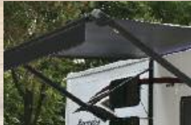
POWER AWNING WITH LED STRIP Extend and retract your awning with the push of a button. Both arms are adjustable to get just the right angle.
