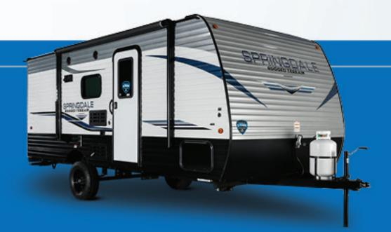
Everything about the new Springdale<sup>™</sup>Rugged Terrain<sup>™</sup> package shouts off-road adventure. Over-slung axles, all-terrain tires, and micro diamond plate skirting deliver increased ground clearance, traction, and durability. Zamp<sup>®</sup> solar prep and a 30 lb. propane tank lets campers go deep into uncharted territory and stay there.
