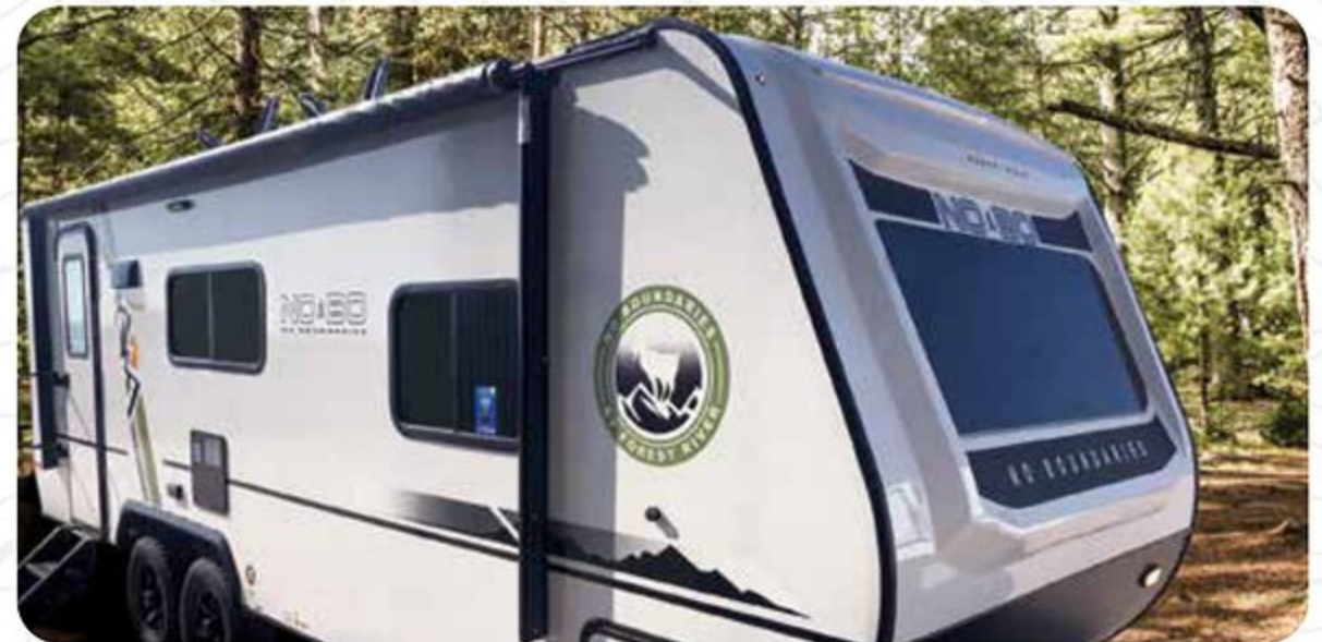
SEAMLESS PANORAMIC FRONT WINDOW 60" X 22" TEMPERED GLASS. FRONT CAP STANDARD WITH BACK COUNTRY PACKAGE ON 19 SERIES, OPTIONAL ON 16 SERIES
