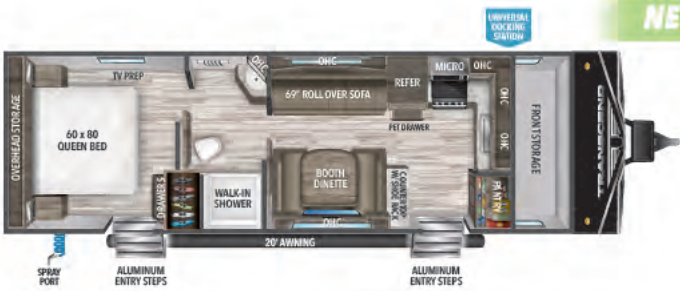
255FK UVW' 5,620 HITCH' 618 LENGTH' 31' 8" HEIGHT 11' 0" CAPACITY 62 68 38
