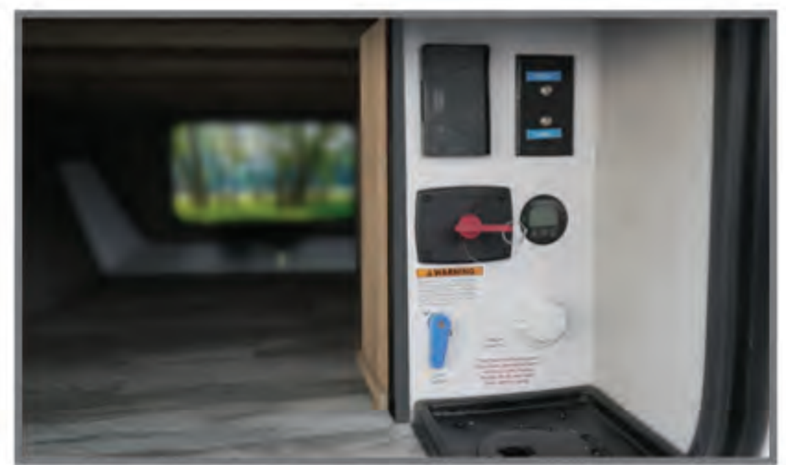
UNIVERSAL DOCKING STATION WITH BATTERY MONITOR
