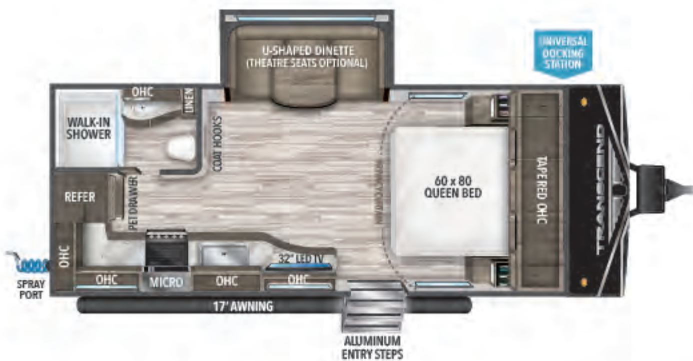
200MK UVW 1 4,796 HITCH 1 480 LENGTH 1 24' 11" HEIGHT 11' 0 CAPACITY 62 39 39
