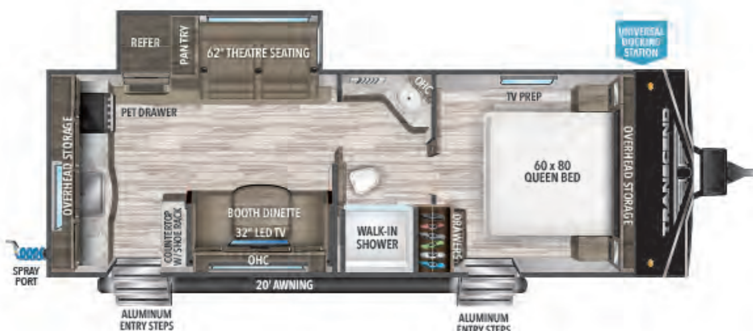
231RK UVW 1 6120 HITCH 1 612 LENGTH 1 29' 3" HEIGHT 11' 0 CAPACITY 62 68 39
