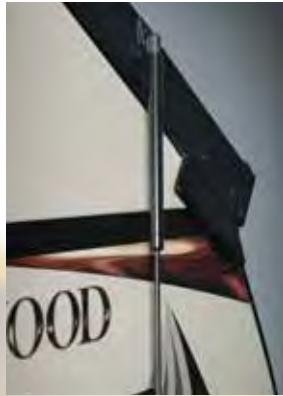
Gas Strut Lift Assist (Std. Hard Side Models w/ Manual Lift Roof Only)
