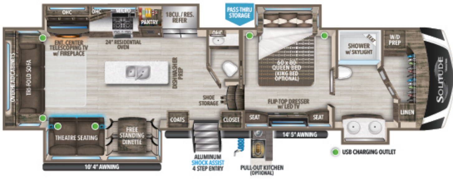
373FB UVW' HITCH' GVWR LENGTH' HEIGHT CAPACITY 373FB-R 13,950 2,800 16,800 41' 4" 13' 5" 81 106 106
