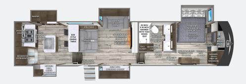
Length: 42'6" Hitch Weight: 3,000 CCC: 3,505 Dry Weight: 14,995 GVWR: 18,500
