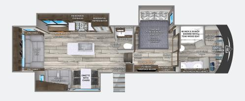
Length: 39'8" Hitch Weight: 3,100 CCC: 1,900 Dry Weight: 14,100 GVWR: 16,000
