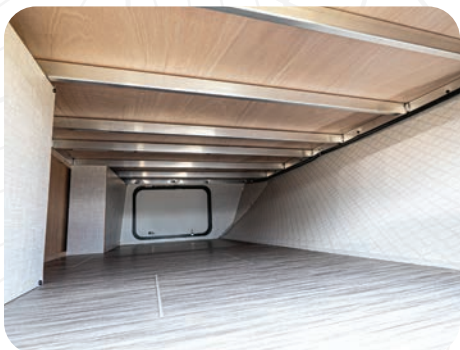
WELDED ALUMINUM BED FRAMING (16/19 SERIES ONLY)
