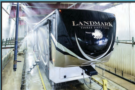
127 SPRINKLER RAIN BAY TEST
