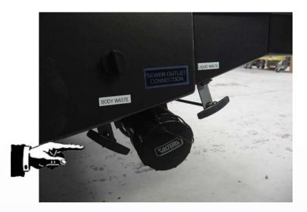
Attach garden hose to the water inlet (located behind the utility access door behind the drivers side rear tires, black cap). Turn on water (from outside source) to spray the interior of the black water holding tank. Continue to leave drain valve open until flushed. Turn off water, disconnect hose and close valve.
