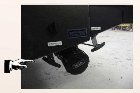
Attach garden hose to the water inlet (located behind the utility access door behind the drivers side rear tires, black cap). Turn on water (from outside source) to spray the interior of the black water holding tank. Continue to leave drain valve open until flushed. Turn off water, disconnect hose and close valve.
