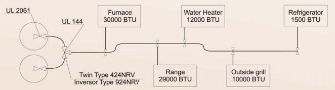
RV installations are supplied by single or double cylinder systems, or by ASME tanks. The integrated second stage regulator is connected to cylinders through flexible high pressure gas rubber hoses, equipped with fittings in accordance to UL 2061 (NFPA 1192; paragraph 5.2.16.4). Installations of integrated double stage regulators have to be in accordance with requirements expressed in NFPA 1192, paragraph 5.2.15.
