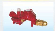
The Two Stage Type 524 AS regulator is mounted directly to tank, connected to the tank valve of ASME container type. It is connected at its outlet to the installation gas pipe net. The regulator inlet POL coupling is equipped with an excess flow valve device.
