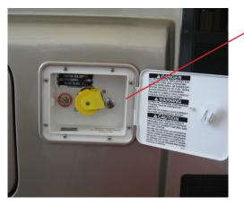
EMERGENCY SHUT OFF: Push in when filling to prevent flow of propane to coach.
