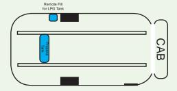
The remote fill valve is located on the utility panel on the driver's side rear compartment. Filling your tank should be done only by a qualified LPG service center.
