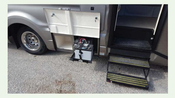
Auxiliary batteries are located next to the Motorhome entry door in a slide out tray. The Lifeline AGM batteries are wired in "series" and will give you over 242 amp hours of use at 12 volts.
