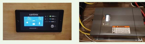
The inverter will supply 110 volt power to the electronic components (Television, DVD player, optional satellite receivers and the electrical outlets when you are not hooked up to shore power or running the generator. These devices will drain your "house" batteries if in use for an extended period of time.
