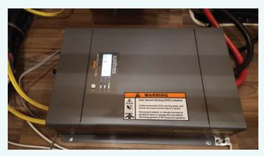
The inverter will supply 110 volt power to the electronic components (Television, DVD player, optional satellite receivers and the electrical outlets when you are not hooked up to shore power or running the generator. These devices will drain your "house" batteries if in use for an extended period of time.
