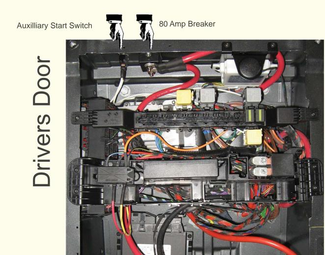
Coach House has added electrical switches / breakers under the Driver's Seat (In the Pedestal). The 80 Amp Breaker and the Auxilliary Start Over-ride switch are located according to the picture above.
