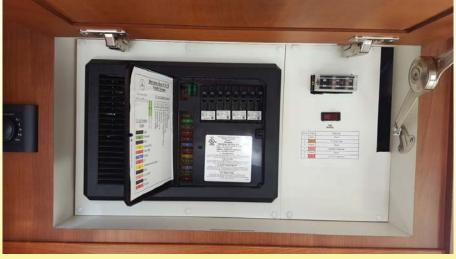
The converter is equipped with an automatic switchover relay to prevent both the generator and the external power cord from being connected to the converter at the same time. When either the external power cord or the generator is being used, both the 110 volt AC system and the 12 volt DC system will be activated inside the motorhome. When neither of these is connected, the 12 volt auxiliary batteries will activate only the 12 volt DC system.
