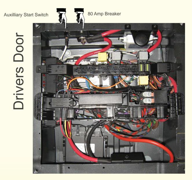
Coach House has added electrical switches / breakers under the Driver's Seat (In the Pedestal). The 80 Amp Breaker and the Auxilliary Start Over-ride switch are located according to the picture above.
