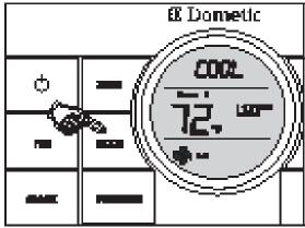
Press the MODE button to cycle through the mode options. A mode is an operation that can be performed by the unit and is controlled by the Dometic CCC thermostat. The available modes are: OFF, COOL, HP (HEAT PUMP), HS (Heat Strip), FAN, FURN (Furnace), and AUTO. The available modes are determined by your system options.
