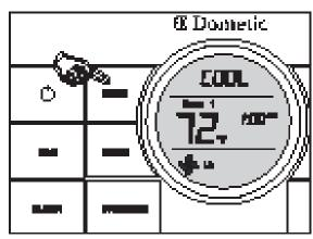
Press the ZONE button to cycle through the available zones to be programmed. Each zone signifies a unit designated to cool or heat a specific area of an RV. The Dometic CCC 2 thermostat can control up to four units (zones).
