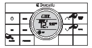
Press the CLOCK button to Initiate the clock setting sub-menu on the CCC 2 thermostat. When entering this menu, the "hour" digits will flash first. Press the CLOCK button again and the "minutes" digits will flash. Press it a third time and the "AM" or "PM" icon will flash.
