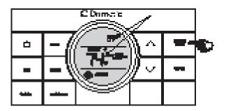
7. Press and hold the INSIDE TEMP button and the LCD will display the current inside temperature recorded at the CCC 2 Thermostat (or at the optional remote indoor temperature sensor) instead of the temperature set-point. The LCD will also display "IN" to indicate that the inside temperature is being displayed. When the INSIDE TEMP button is released, the LCD will return to the programmed temperature set-point.
