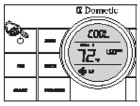
To turn ON the CCC 2 thermostat when the back light is off, first press any button to wake up the CCC 2 thermostat. Then press and release the ON/OFF button.
